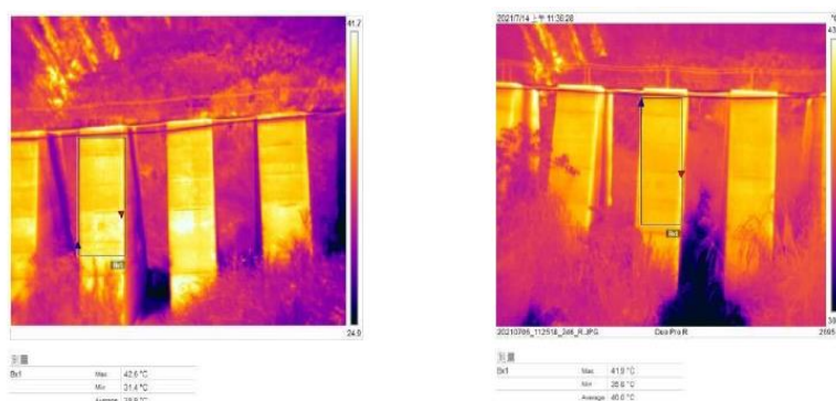
Figure 9: Use FLIR TOOL to analyze the thigh-low emperature difference in Area A
